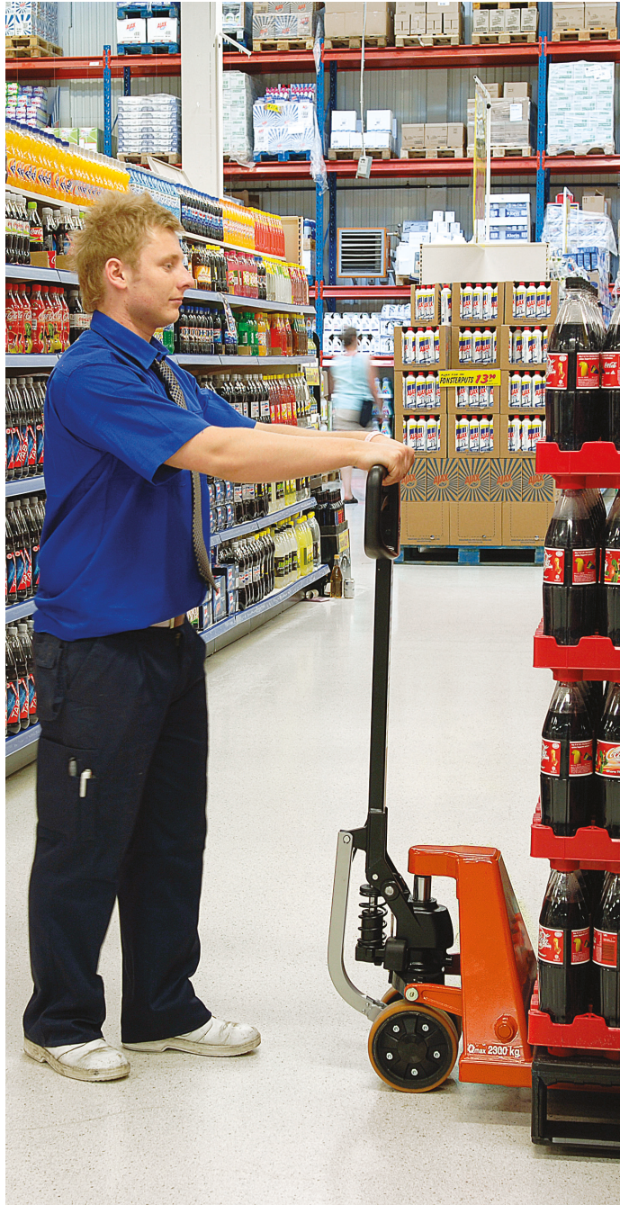
The LHM230P's steering arm provides leverage to the wheels to help get the truck moving
