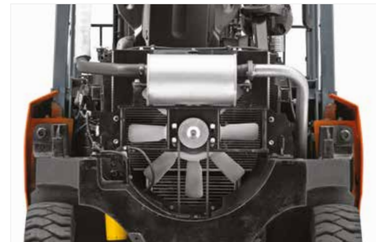
Highly effective cooling systems ensure consistent performance in all environments
