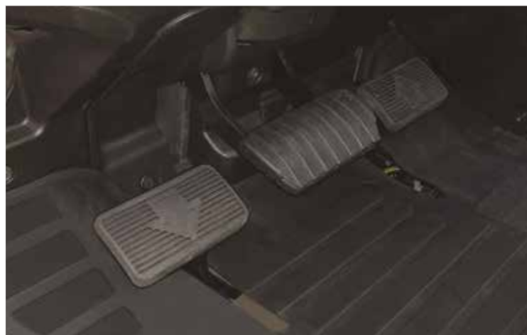
Choice of pedal layouts to suit any application (double pedal layout shown)
