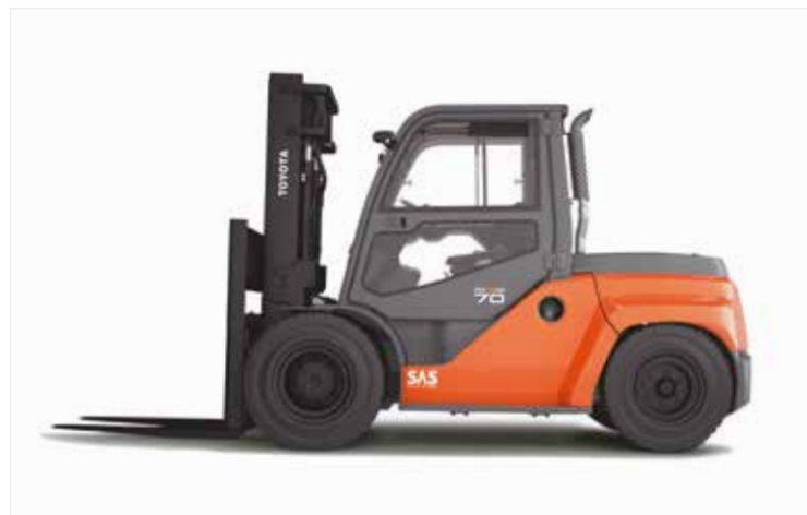
Steel cabin option offers a high comfort level in all weather conditions
