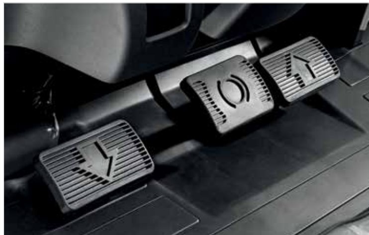
Different pedal layouts to suit driver preference. (Double pedal layout option shown)
