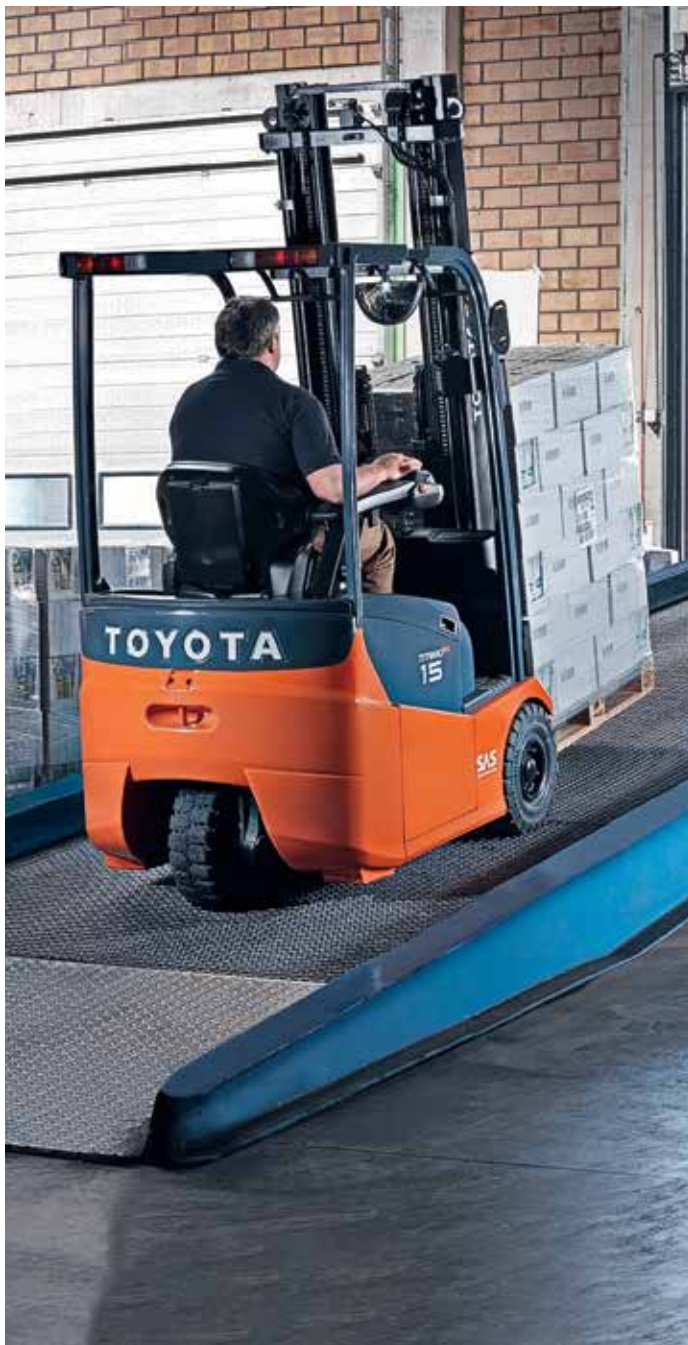
The clear-view mast gives operators an excellent view to the load and working environment.
